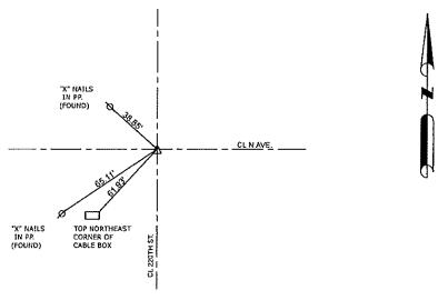
ALL TIE DISTANCES ARE MEASURED HORIZONTALLY USING GPS
