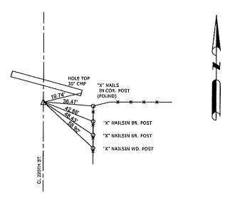
ALL TIE DISTANCES ARE MEASURED HORIZONTALLY USING GPS
