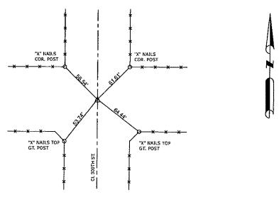
ALL TIE DISTANCES ARE MEASURED HORIZONTALLY USING GPS
